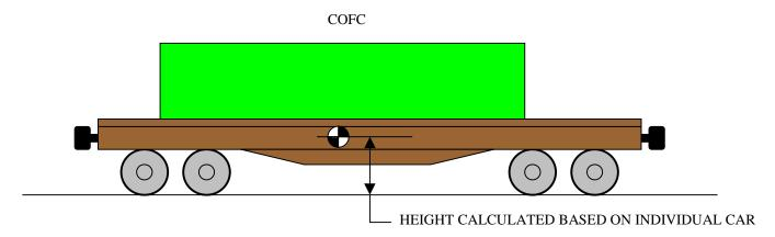
Center of gravity should not exceed 98" at top of rail (ATR). In some cases it can exceed 98" ATR to a maximum of 110" ATR, however, the 110" maximum restricts train handling and operations. You may use the following information to figure it:
